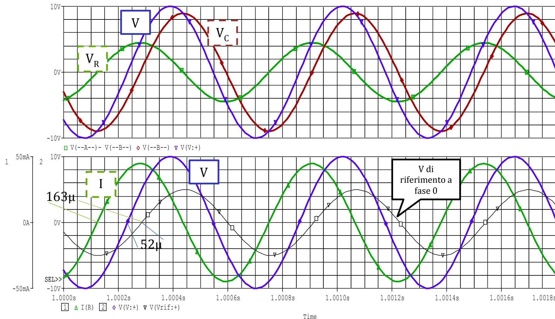
$$\frac{t}{T} = \frac{\alpha}{2\pi} \rightarrow t = \frac{\alpha}{2\pi} \cdot T = \frac{\alpha}{2\pi f} = \frac{\alpha}{\omega} \rightarrow \begin{cases} \alpha = \frac{\pi}{6} (30^\circ) \rightarrow t = \frac{\frac{\pi}{6}}{10k} \cong 52,4 \mu s \\ \alpha = 2,93 \text{ rad} \rightarrow t = \frac{1,63}{10k} \cong 163 \mu s \end{cases}$$
